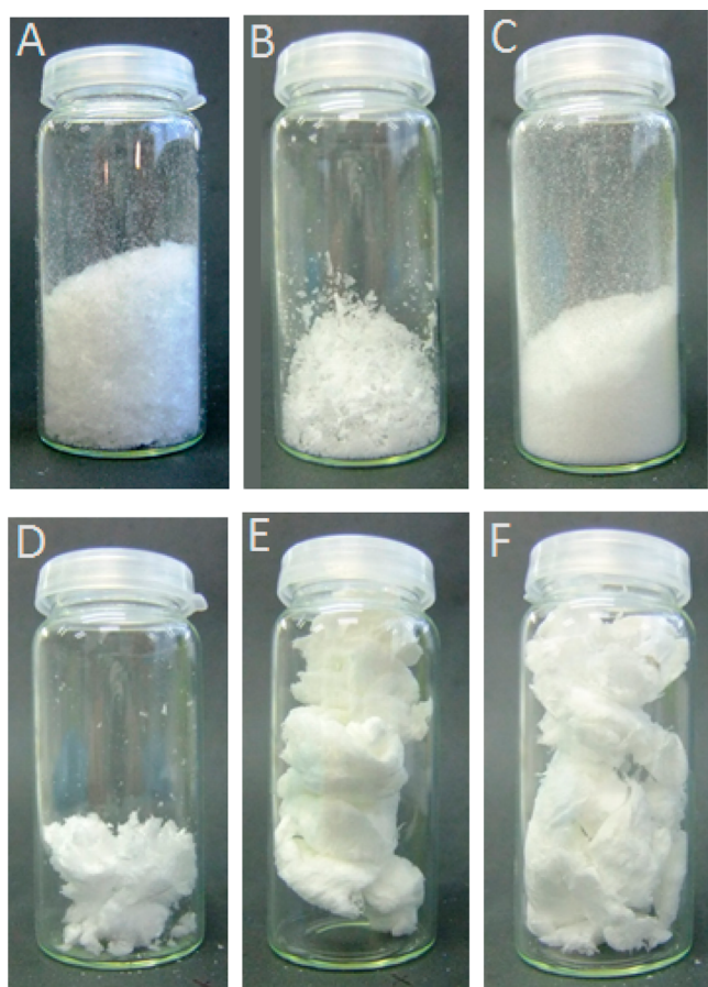
Figure 4. Appearance of freeze-dried cotton CNC samples consisting of (A) unmodified CNC, and a 50:50 mixture using (B) PEO 0.0015 M, (C) PEO 0.0034 M, (D) PEO 0.035 M, (E) PEO 0.1 M, and (F) PEO 5 M.
